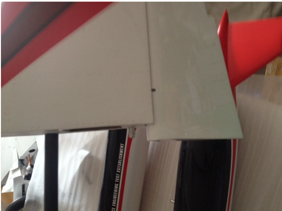
Photo 4 – additional front screw to the front pin of the vertical stab.
