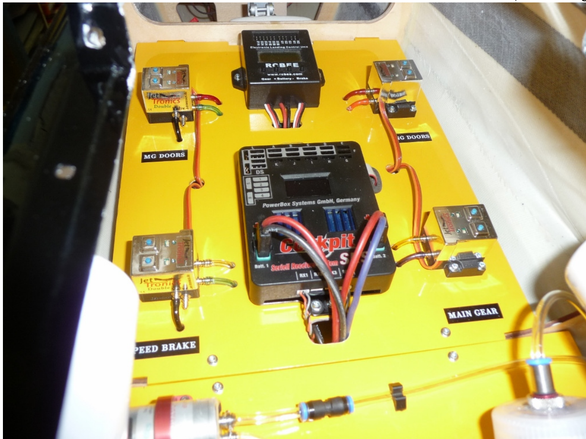
Photo 2 – air lines colour coded and run to the centre area of the component boards. The Speed brake air lines have been run to this spot too.
